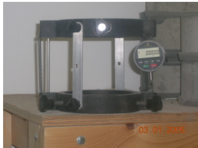
Figure 3. 2: Compressometer used to measure Elastic Modulus
