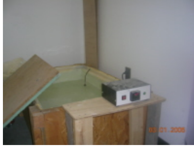
Figure 3. 1: Curing Bath with OMEGA temperature controller
