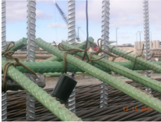
Figure 3. 6: Intellirock data logger attached to confining steel (location 5) at the end of the girder.
