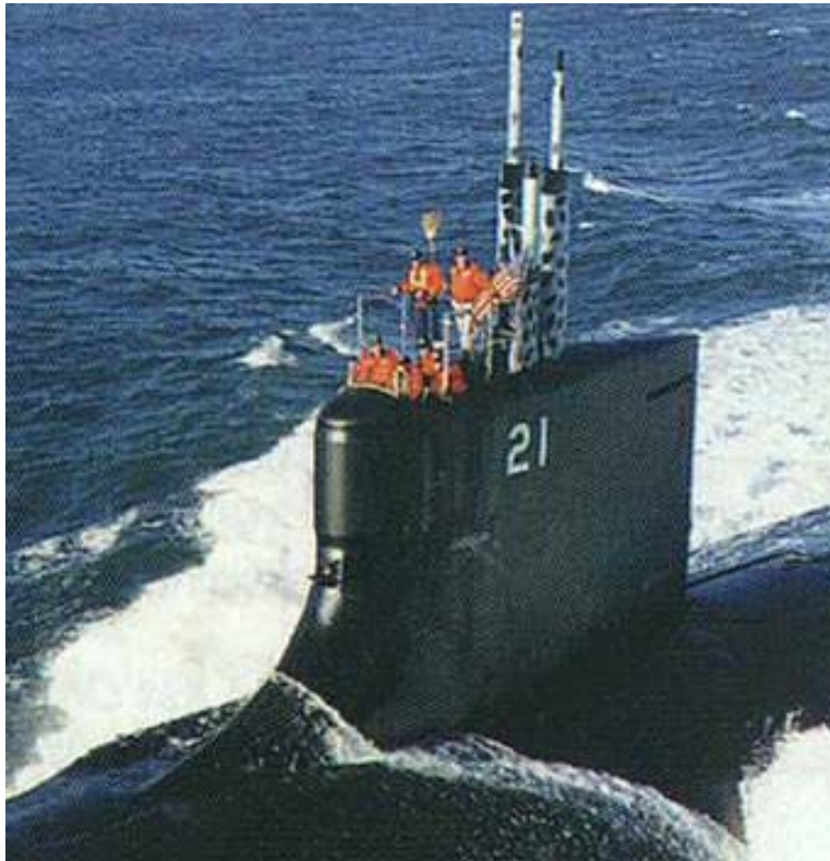
Figure 2.11 Fillet on the leading edge of a Seawolf class submarine conning tower.
