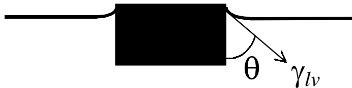
Figure 2-3. Common misconception of three-phase contact with cubical particle.
