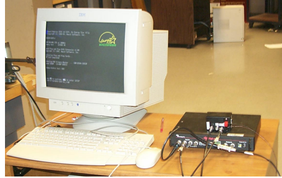
Figure 2.14 Low-cost impedance box, SigLab Analyzer and PC
