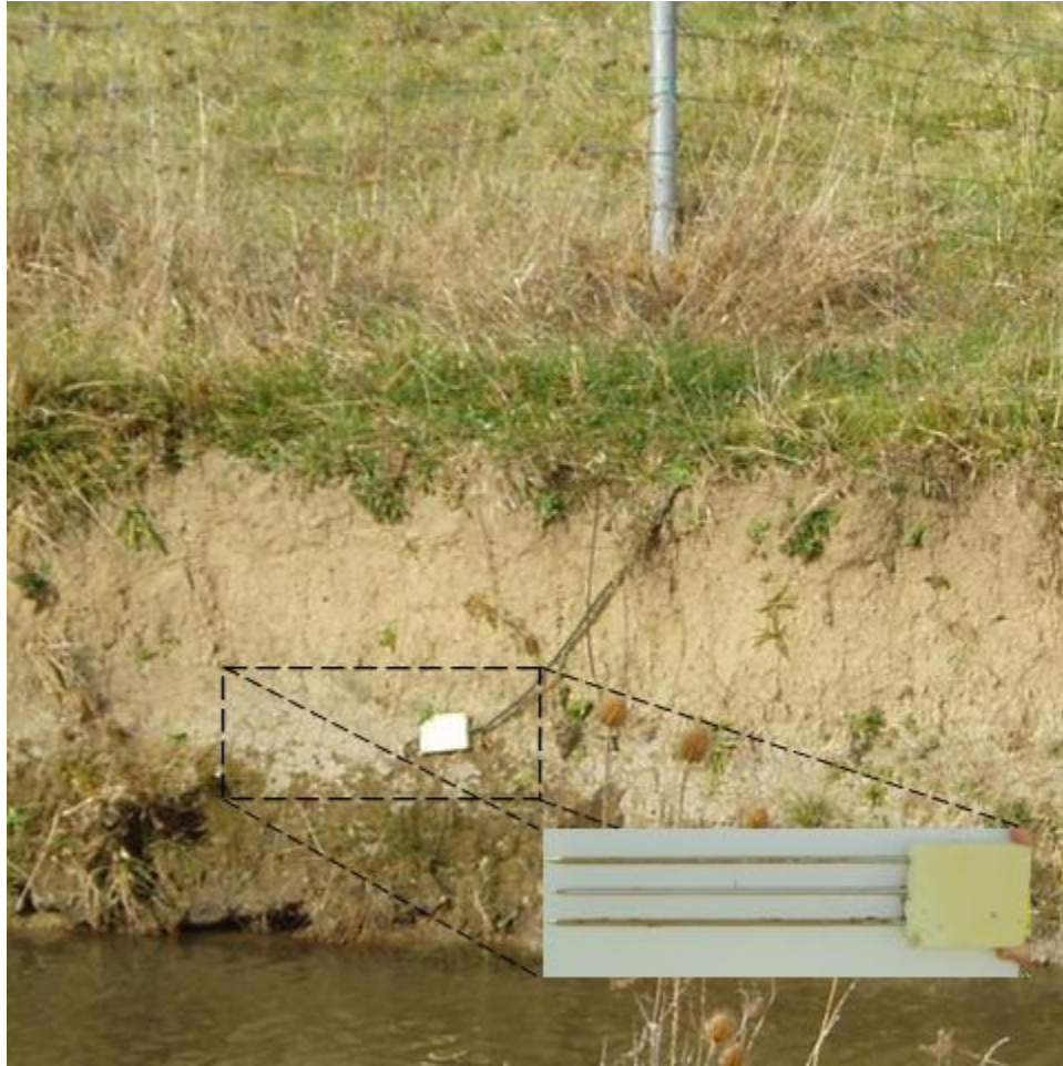
Figure 10 View of TDR probe inserted into streambank.
