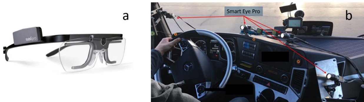
Figure 4. a) Tobii Glasses 2 head-worn eye-tracker ( https://www.tobiipro.com/product-listing/tobii-pro-glasses-2/ ) b) Smart Eye Pro remote eye-tracking cameras; Adapted from (Lotz et al., 2020)
