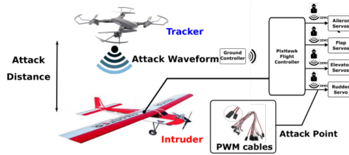
Figure 2.10: The attack scenario includes two UAVs, namely an intruder and a tracker. The tracker uses FAI to block or manipulate the actuation control of the intruder to defend the safe air-space.
