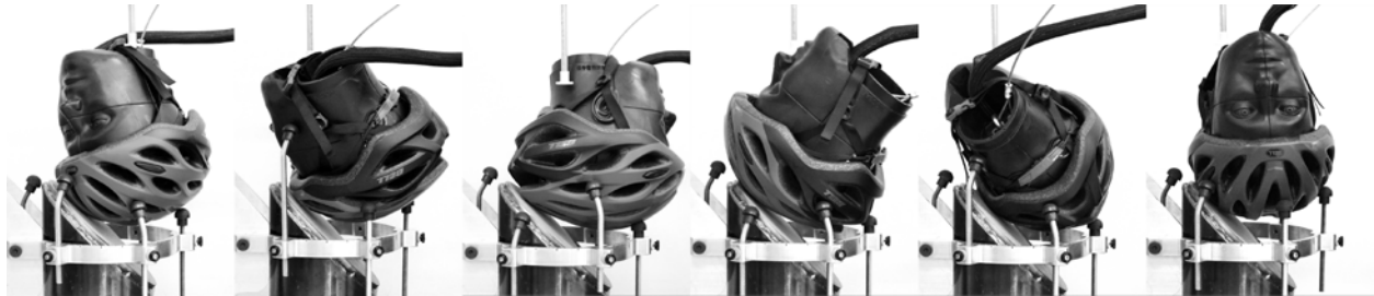
Figure 2. Impact locations 1-6 (left to right). Locations 1, 2, and 6 represent body-driven impacts, in which the head leads the body, locations 3 and 5 represent skidding-type impacts, and location 4 represents an impact from flipping over the handlebars.
