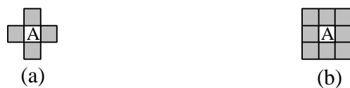
Figure 2.1 Connectivity on a grid. A pixel is said to be 4- or 8- connected if it has the same properties as one of its nearest four or eight neighbors. Pixel A and its (a) 4-connected and (b) 8-connected neighbors
