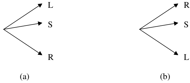
Figure 2.12: Lax shock condition for traffic flow problem: (a) not a shock, (b) shock
