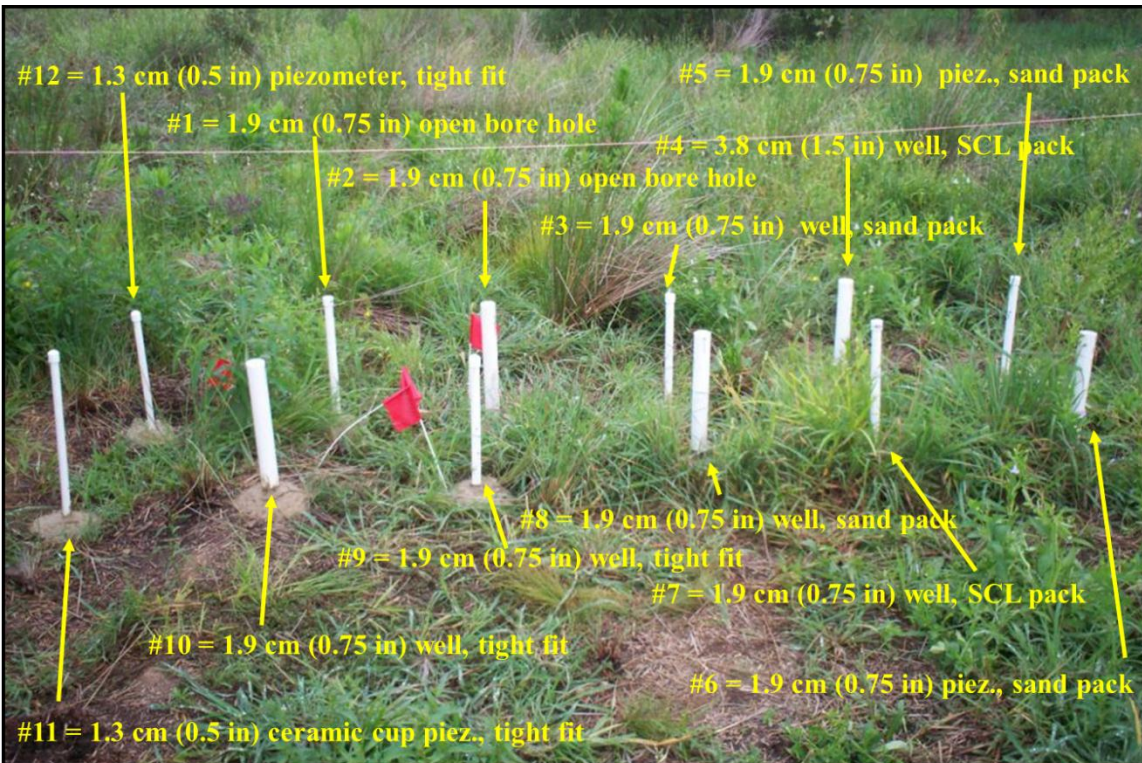
Figure 14. Layout and description of the various types of the manually monitored wells and piezometers at the Cedar Run Site.
