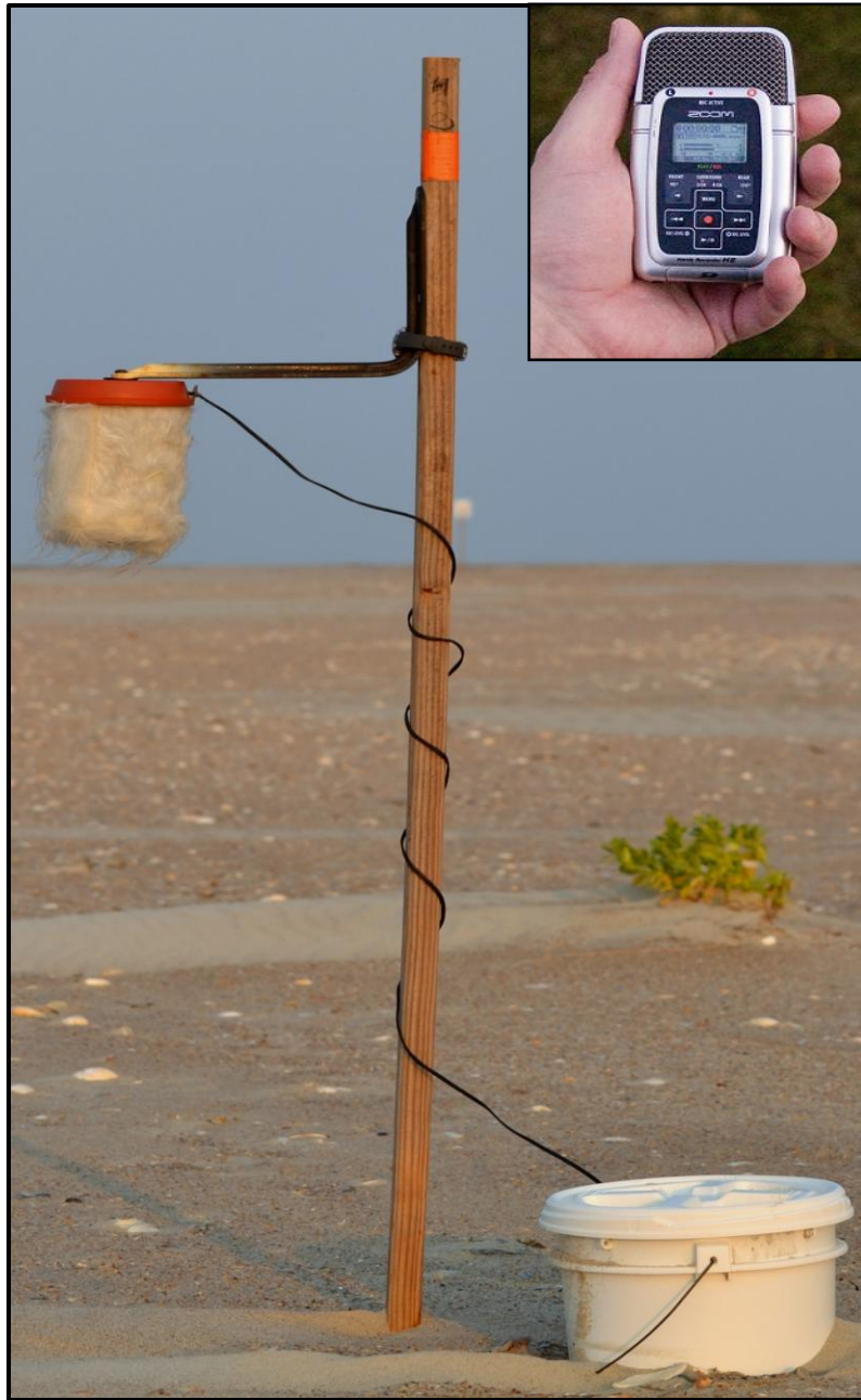
Figure C2. Audio-monitoring methods: Weather-proofed Zoom H2 Digital Audio Recorder connected to a 12 V sealed lead-acid battery (in bucket) with close-up of recording unit. These units recorded within-colony sound environments continuously for 24 hr/day throughout the 4-month nesting seasons in 2010-2011.
