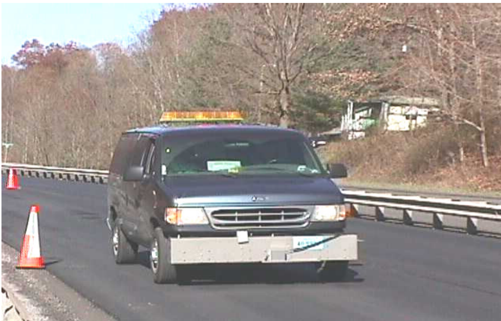
Figure 2-4 VDOT Laser Profiler on Route 460 in Tazewell, Virginia
