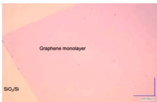
Fig. 3. Graphene monolayer transferred onto SiO_2/Si following the procedure outlined in the text.
