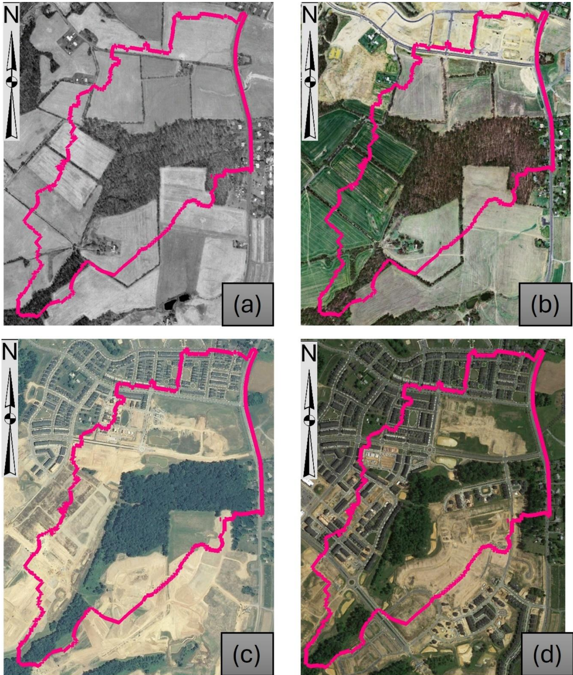
Figure 1-3. Satellite imagery of Trib 109 during the year of a) 1993, b) 2006, c) 2011 and d) 2013. The red line indicates the catchment boundary following development.
