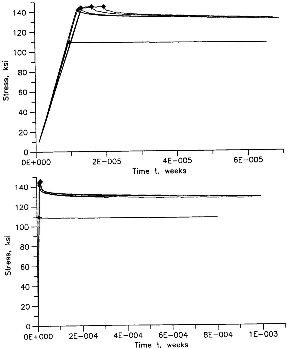
Figure 17. Static relaxation Ti-6Al-4V
