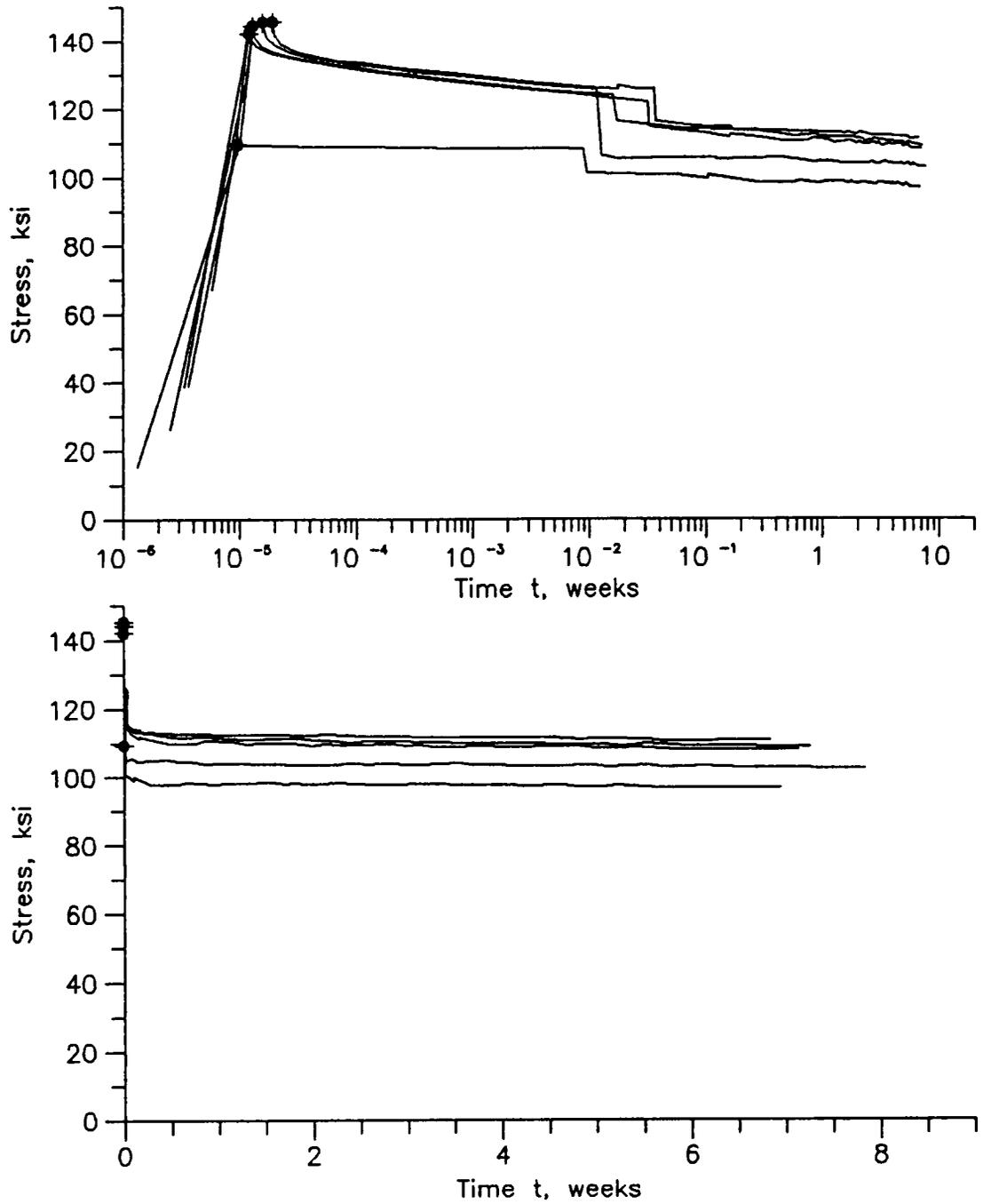
Figure 16. Static relaxation Ti-6Al-4V
