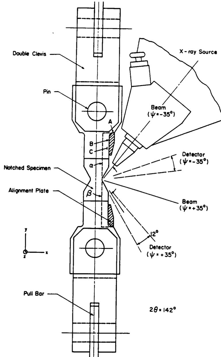
Figure 39. Arrangement of specimen, fixtures, and x-ray source, for measurements during mechanical testing.
