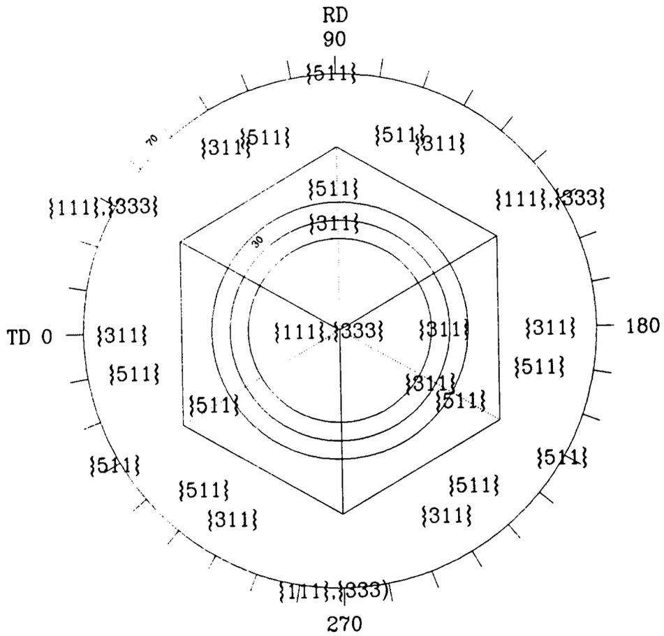
Figure 28. Aluminum crystal orientation and reflections pole figure, cubic crystal.
