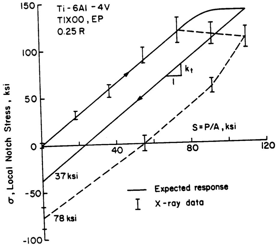
Figure 41. Agreement of x-ray stress with Neuber's estimate for notched Ti-6Al-4V.
