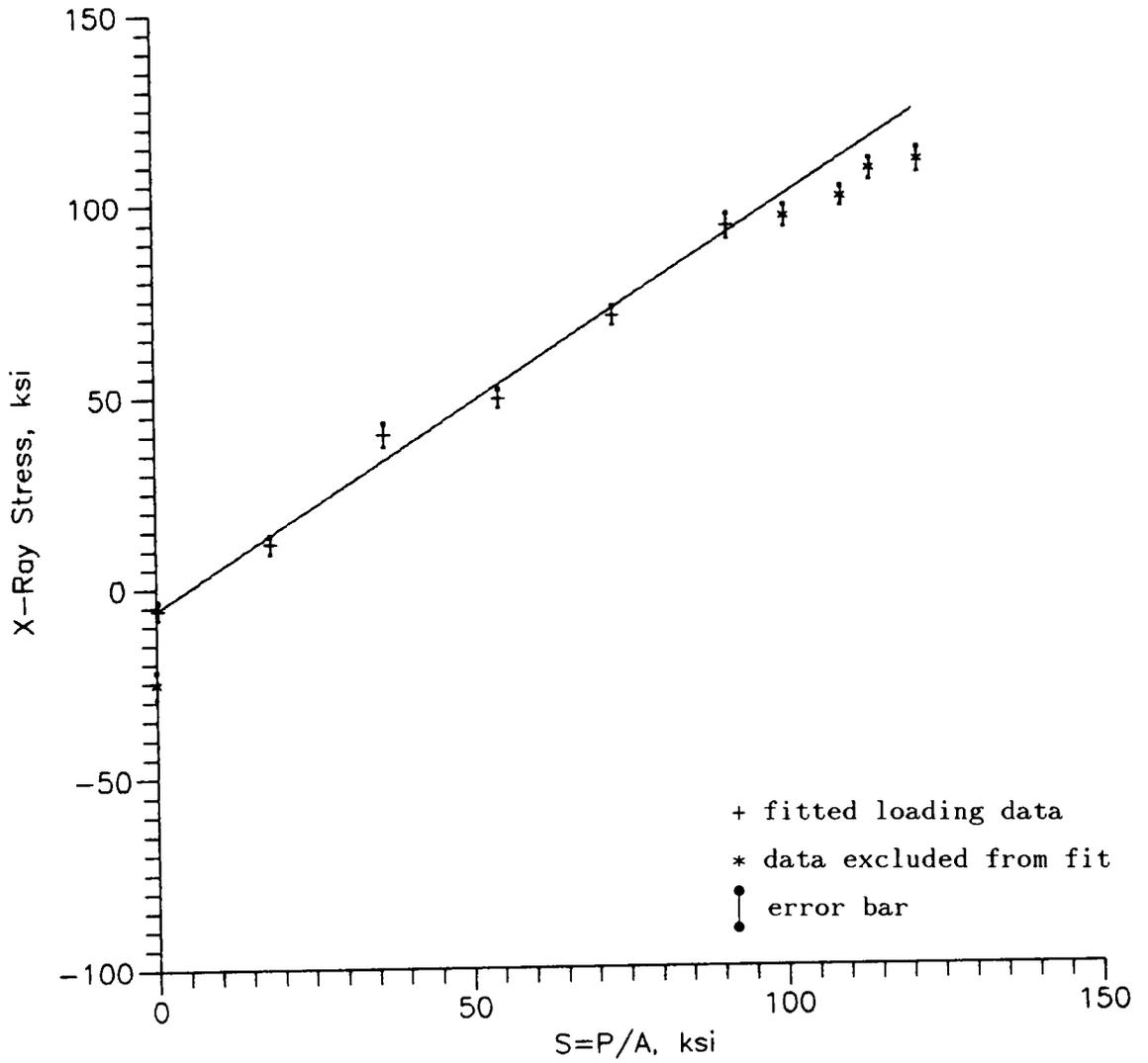
Figure 19. Agreement of x-ray with P/A for unnotched Ti-6Al-4V, specimen T1S02.
