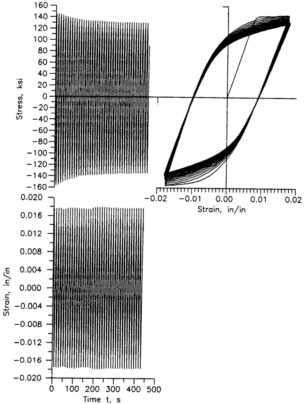
Figure 2. Cyclic softening Ti-6Al-4V.
