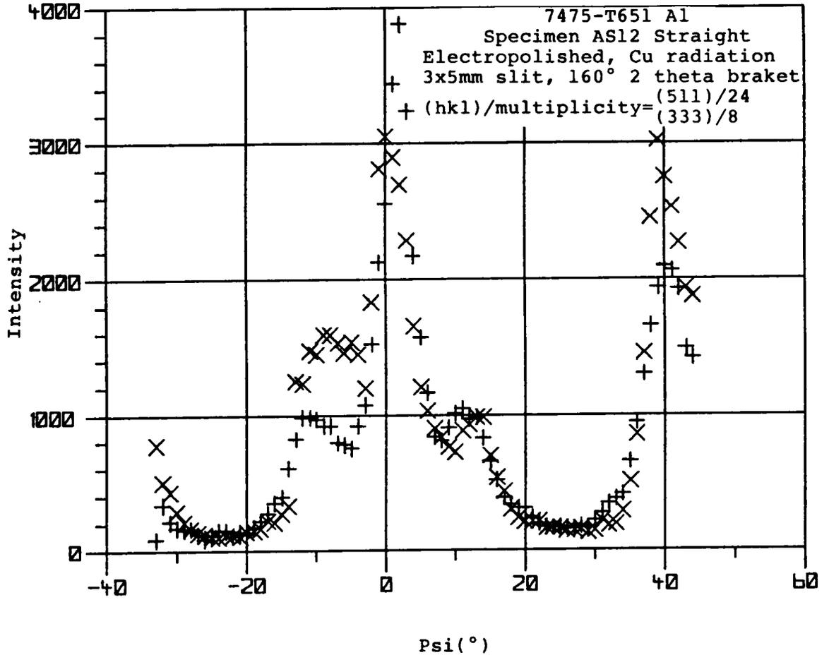
Figure 29. 7475-T651 Al intensity variation on the x-ray stress analyzer, for a large number of measurements.
