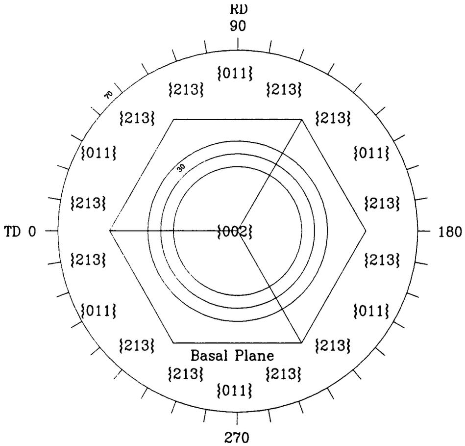
Figure 34.  $\alpha$ -Titanium crystal orientation and reflections pole figure, hcp crystal,  $a=2.950 \text{ \AA}$ ,  $c=4.686 \text{ \AA}$ .
