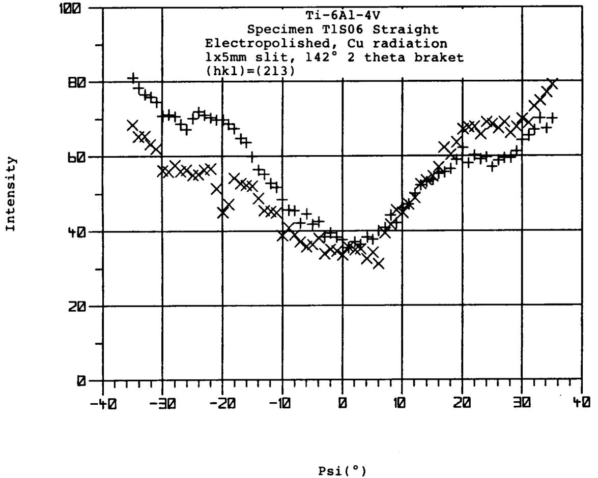
Figure 35. Ti-6Al-4V intensity variation on the x-ray stress analyzer, for a large number of measurements.
