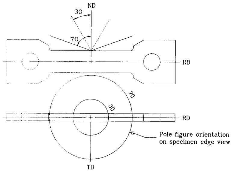
Figure 22. Pole figure and x-ray sample orientation.
