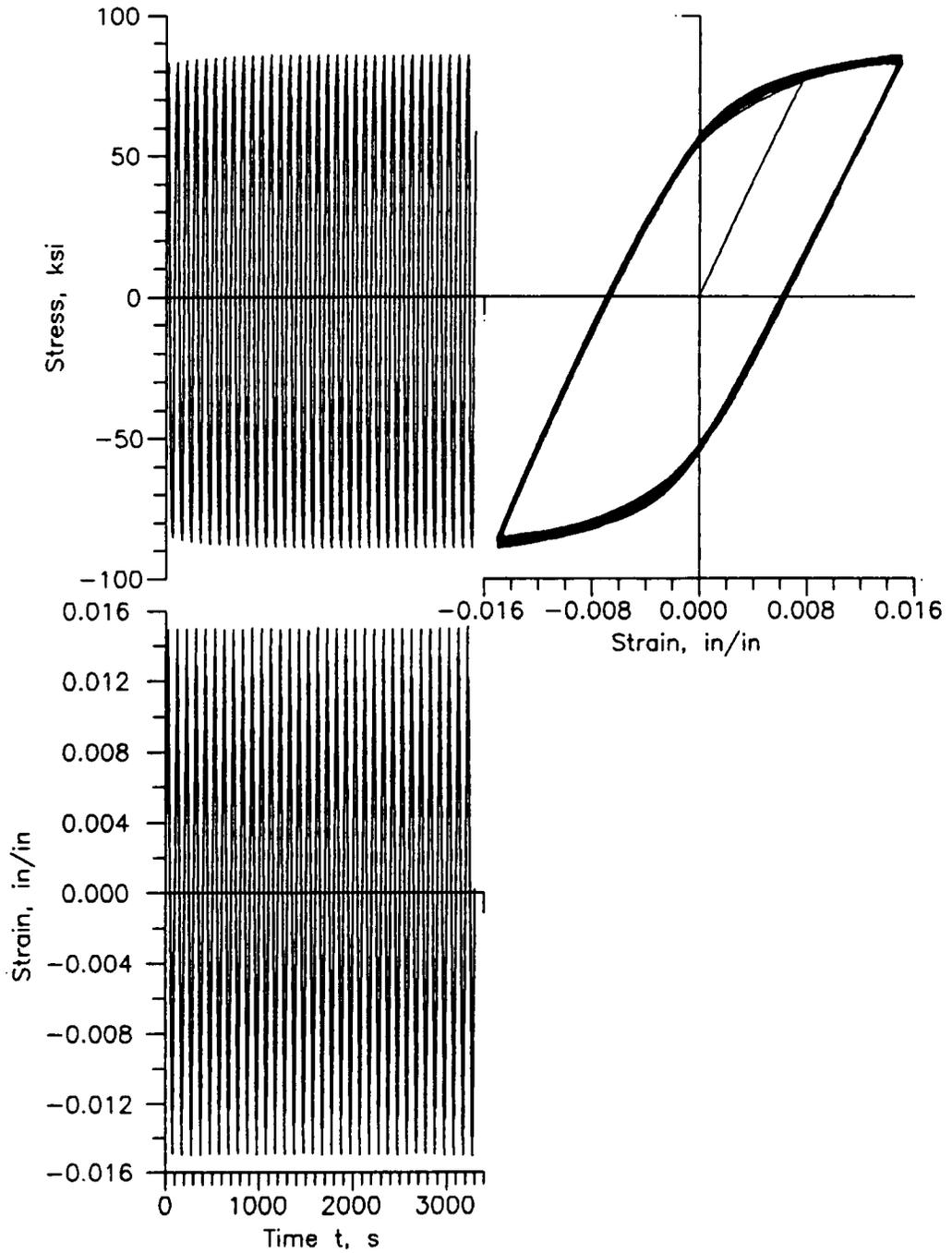
Figure 1. Cyclic hardening 7475-T651 Al,
