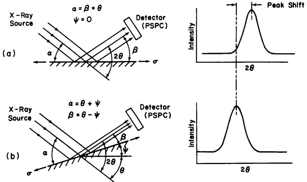
Figure 6. Residual stress measurement by x-ray diffraction.
