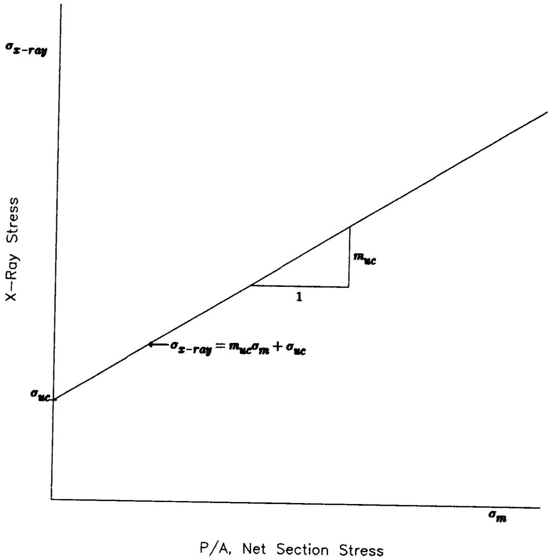
Figure 21. Illustration of x-ray stress versus  $P/A$ .
