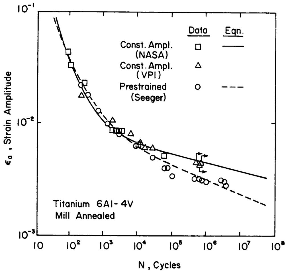
Figure 10. Strain Life Curve Ti-6Al-4V.
