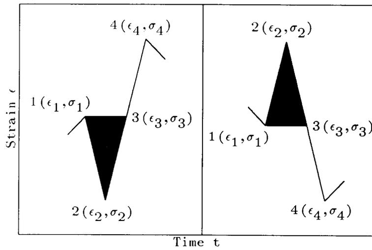
Figure 9. Representative strain counted cycles.
