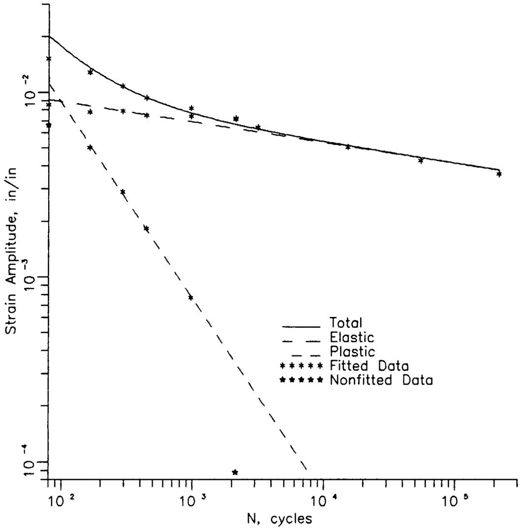
Figure 11. Strain Life Curve 7475-T651 Al.
