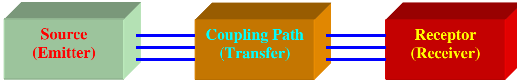
Figure 1-1 Conducted EMI Emission Illustration
