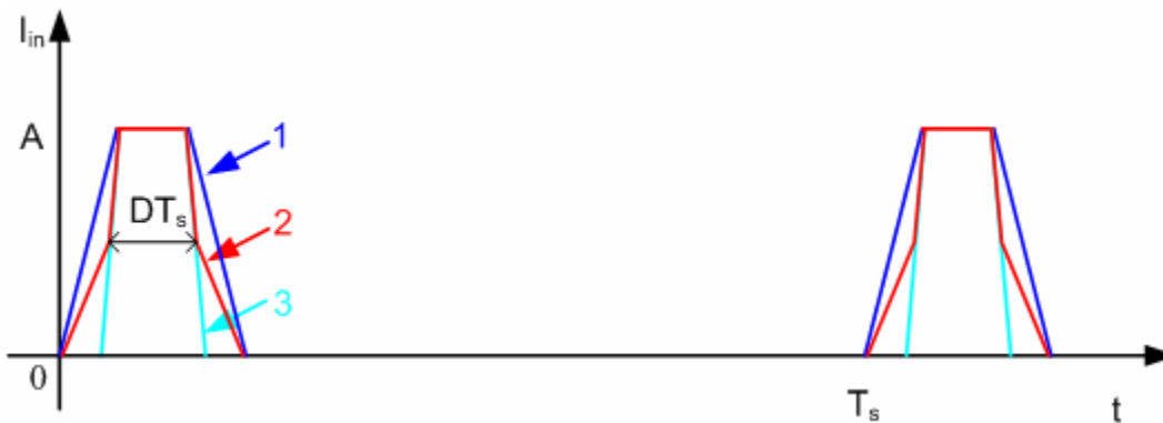
Figure 2-9 Multi-slew-rate Time-domain Waveform
