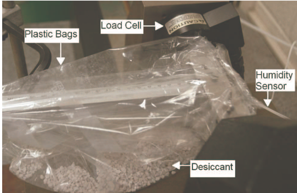
Figure 5.2: Photograph of a PF-SYP DCB fracture specimen inside two plastic bags mounted in the cyclic testing system, with desiccant, humidity sensor, and load cell indicated.
