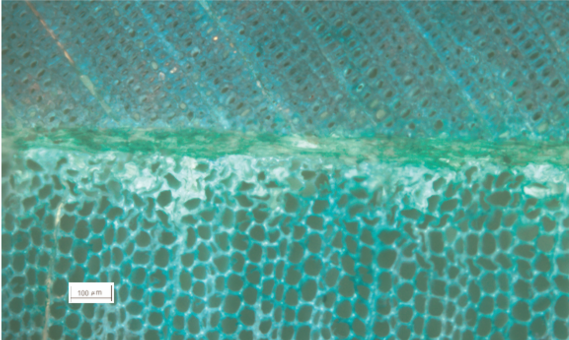
Figure 1.7: Photomicrograph of microtomed cross-sections of a PF bond, showing collapsed earlywood cells.
