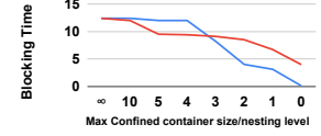
Figure 3. Application blocking time by setting different thresholds for container size and nesting level.
