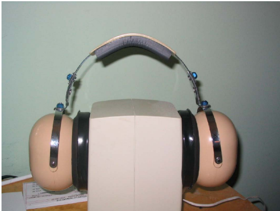
Figure 3.1: DCCI 9AN/2 ear cup with DCCI undercut seals
