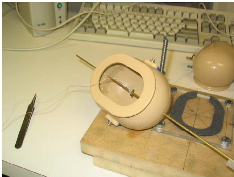
Figure 4.24: Picture of test set up for mode shape identification
