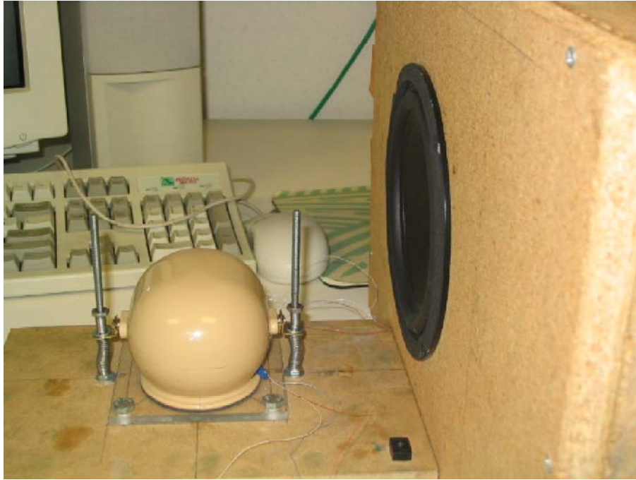
Figure 4.5: Set up of Helmholtz tests
