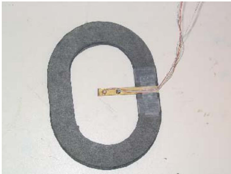
Figure 4.31: Picture of velocity probe and seal
