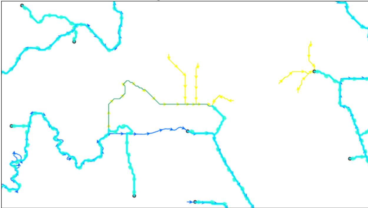
Figure A3. A map showing that there may exist flowlines that do not agree with the NHD despite being made directly from the flow accumulation provided with the NHD flowlines. This needs to be selected by hand.
