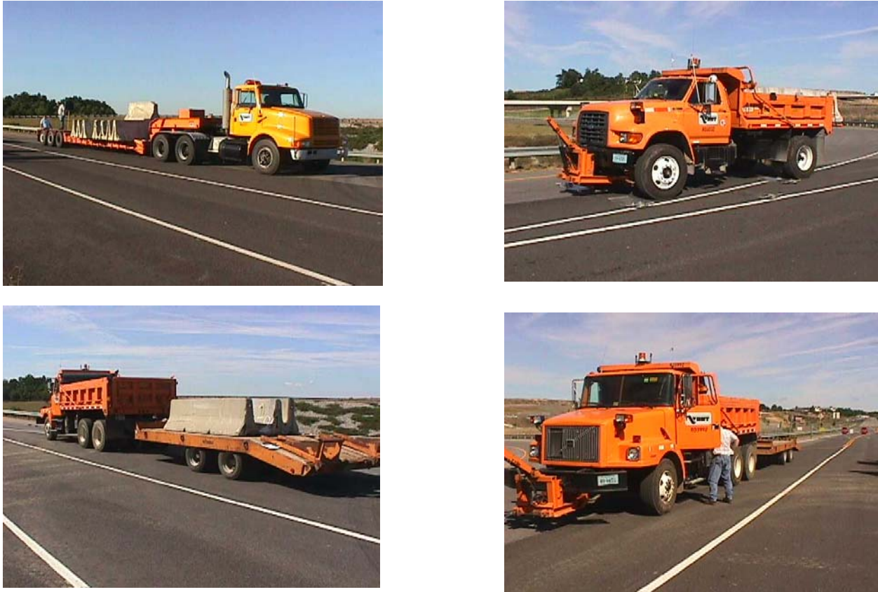
Figure 3-1 - Test vehicles: 6-axle tractor trailer (top left); 2-axle dump truck (top right); 3-axle dump truck with equipment trailer (bottom left); 3-axle dump truck (bottom right)
