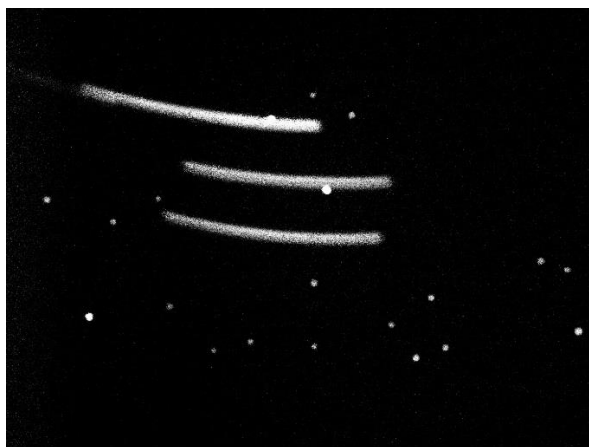
Figure 4.1. These fluorescent images are from CHO-K1 cells labeled with Calcein green AM inside microfluidic channel. (a) Flow rate is 50 \mu\text{l}/\text{min} and UV light exposure time is 7 ms. (b) Flow rate is 100 \mu\text{l}/\text{min} and UV light exposure time is 7 ms.
