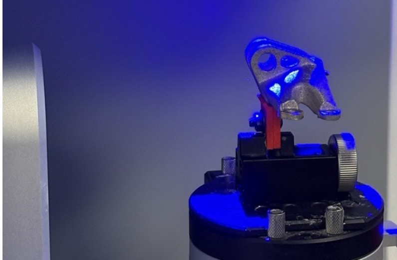
Figure 3-10: As-printed bracket during 3D scanning.
