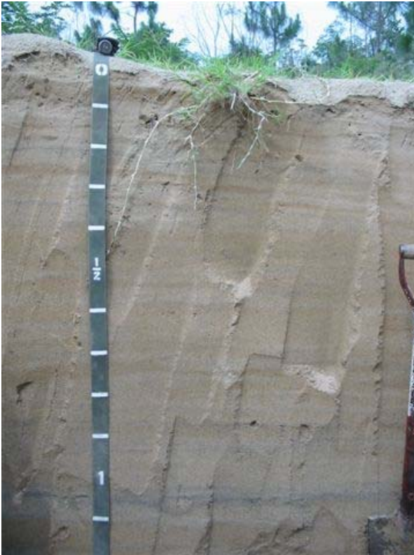
Figure 4. Stratified sandy dredge materials and surface soil at the WWMS site before excavation. Photographed by Lee Daniels, used with permission
