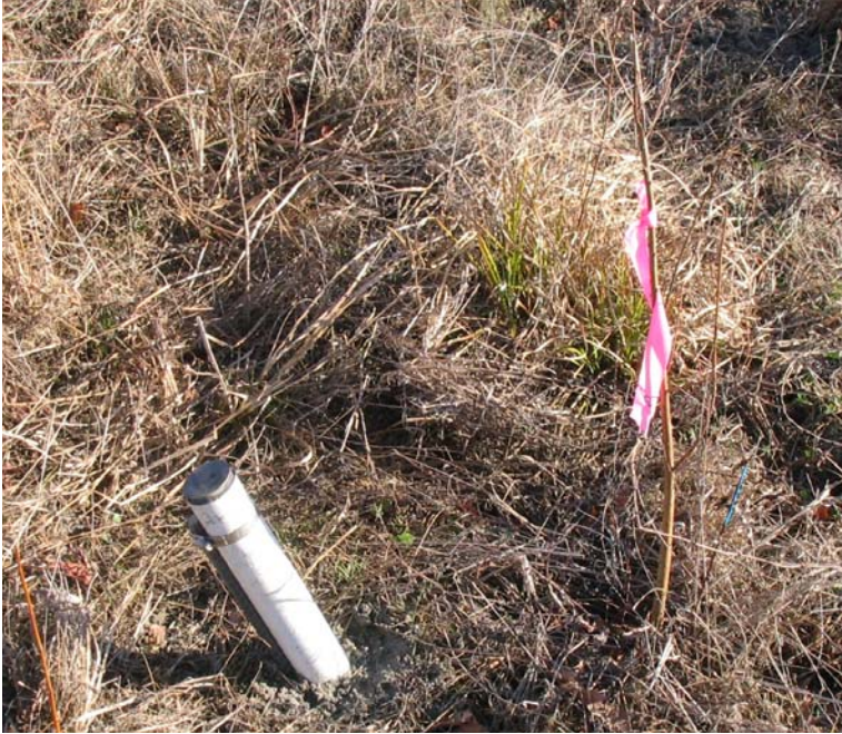
Figure 16. Photograph of an installed CAB tube, February 24, 2006. Photograph by author.
