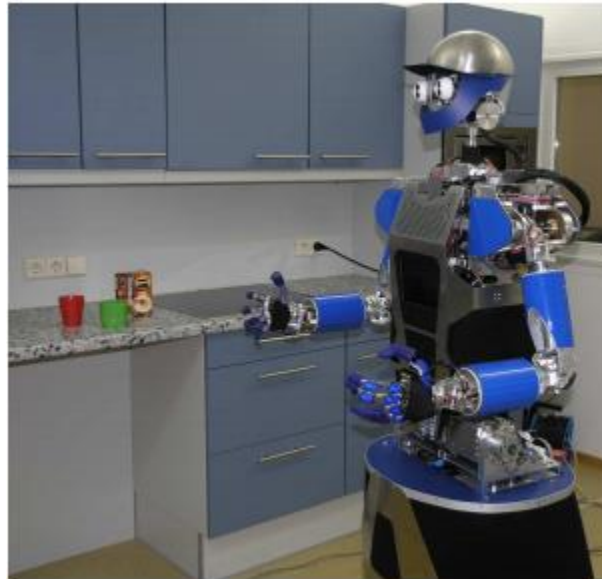
Figure 3.2 ARMAR III home assistant robot with mobility base and vision system. Under fair use policy (T. Asfour, et al., 2006).
