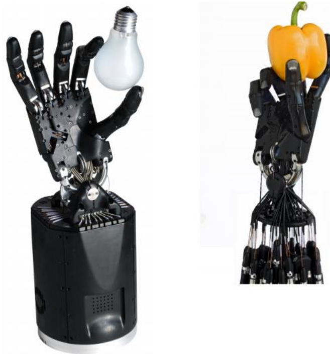
Figure 2.6 Shadow smart motor platform (left) and Shadow air muscle platform (right) holding objects with its dexterous 24 DOF hand. Under fair use policy (Shadow, 2013).
