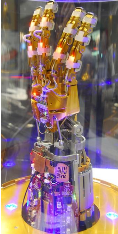
Figure 2.5 Robonaut 2 extrinsically actuated humanoid hand with force sensors around each finger link. Under fair use policy (Guizzo, 2012).
