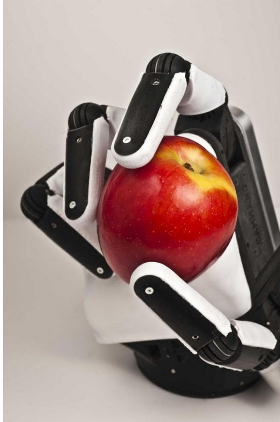
Figure 2.3 Sandia National Labs intrinsic hand with modular fingers attached to a palm platform. Under fair use policy (Hobby, 2012).
