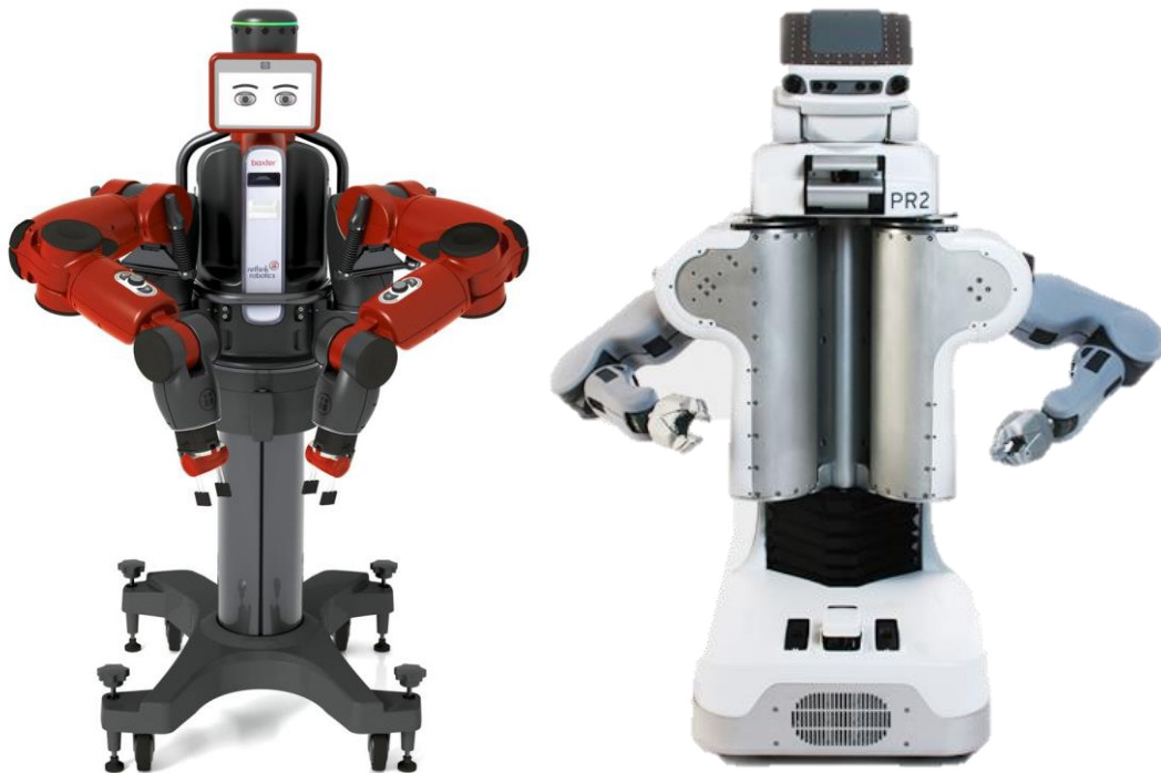
Figure 1.1 Baxter the stationary robotic assembly line worker (left) and the PR2 research platform capable of dynamic localization and navigation (right). Under fair use policy (Deyle, 2012) and (Garage, 2012)
