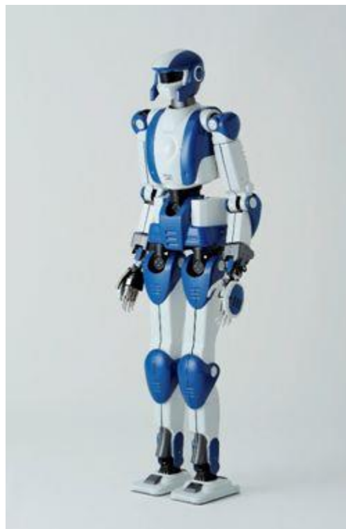
Figure 3.1 HRP-4 Robot with 34 DOF and each arm weighing 0.5kg. Under fair use policy (AIST, 2011)
