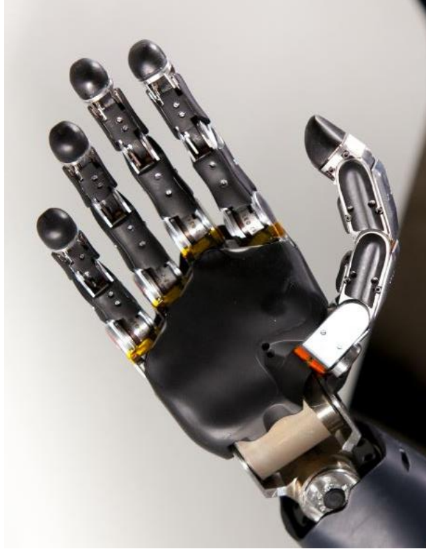
Figure 2.2 Prosthetic hand designed by Kinea with motors at each joint and a multitude of sensors for sending information to user's nervous system. Under fair use policy (Kinea, 2009).
