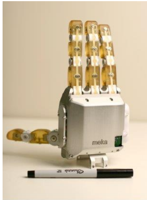
Figure 2.1 The 3 fingered Meka intrinsic hand is fully modular at the wrist with self-contained electronics for use on a separate robotics system. Under fair use policy (Meka, 2009)
