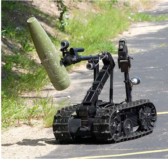
Figure 1.3 Talon robot from QinetiQ moving an IED shell (left) and The Protector by HDT with the modular mini-flail attached (right). Under fair use policy (Annear, 2013) and (Magnuson, 2012)
