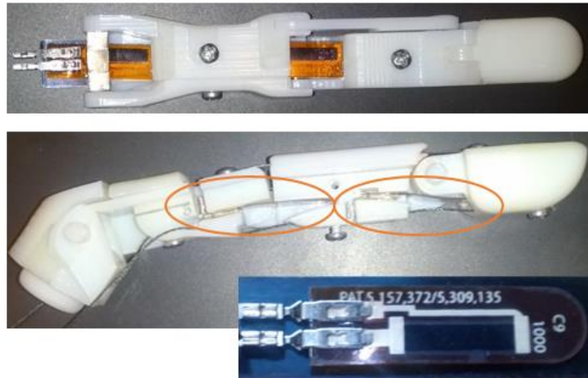
Figure 2.14 Bend sensor shown against a piece of spring steel measuring 32mm x 8mm in length and width. The metal connectors can be bent vertically for installing into the finger system
