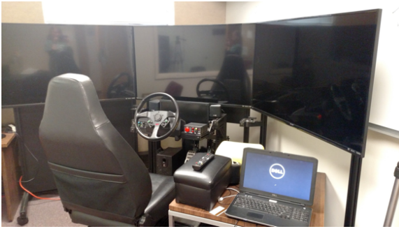
Figure 1: NADS MiniSim Driving Simulator.
