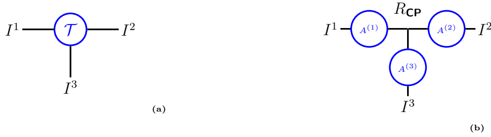
Figure 1.2: a. Graphical representation of an order-3 tensor; b. Graphical representation of a CP decomposition of an order-3 tensor
