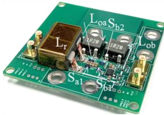
Fig. 4-10. Prototype of the Series-Resonator Buck (SRB) converter using the design procedure in Fig. 4-9, the specifications in Table 4-2, and the component values in Table 4-3.
