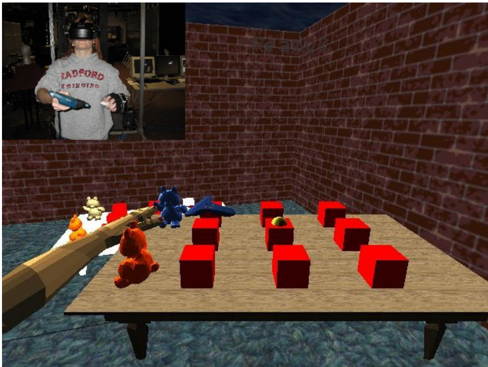
Figure 12: The following sequence of screenshots shows a user performing a manipulation with the Voodoo Dolls redesign. In the first and second pictures, they are creating the manipulation context. The last screenshot demonstrates how the user can manipulate objects on the left side of the context without crossing her hands.
