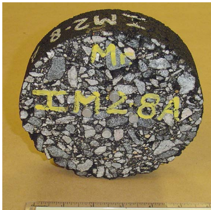
Figure 3-2. Typical specimen for IDT creep compliance test.
