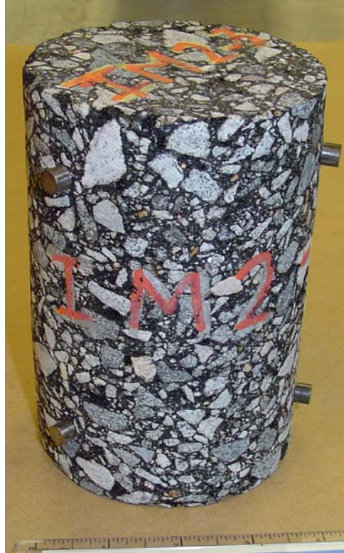
Figure 3-1. Typical specimen for uniaxial creep compliance and dynamic modulus test.
