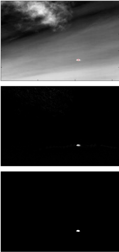
FIGURE 6: PROOF OF CONCEPT FOR AUTOMATED IR CAMERA TARGET DETECTION. FROM TOP TO BOTTOM: RECORDED IMAGE (X MARKS TARGET), IMAGE WITH MEAN REMOVED, BINARY THRESHOLDED IMAGE.
