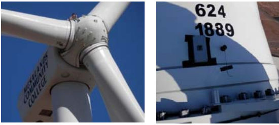
FIGURE 1: (L) THE NAWRTC WIND TURBINE (R) ATTACHMENT CONFIGURATION FOR THE SENSORS ON THE BLADE
