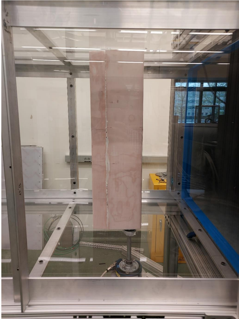
Figure 39. Side view of the 3D printed mount placed in Goodwin 140 closed section wind tunnel.
