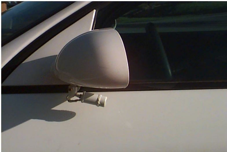
Figure 3.7. Camera Mounted Under the Side Mirror.
