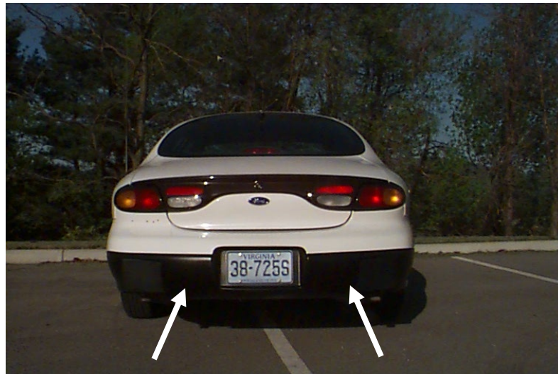
Figure 3.12. Rear Radar Units.
