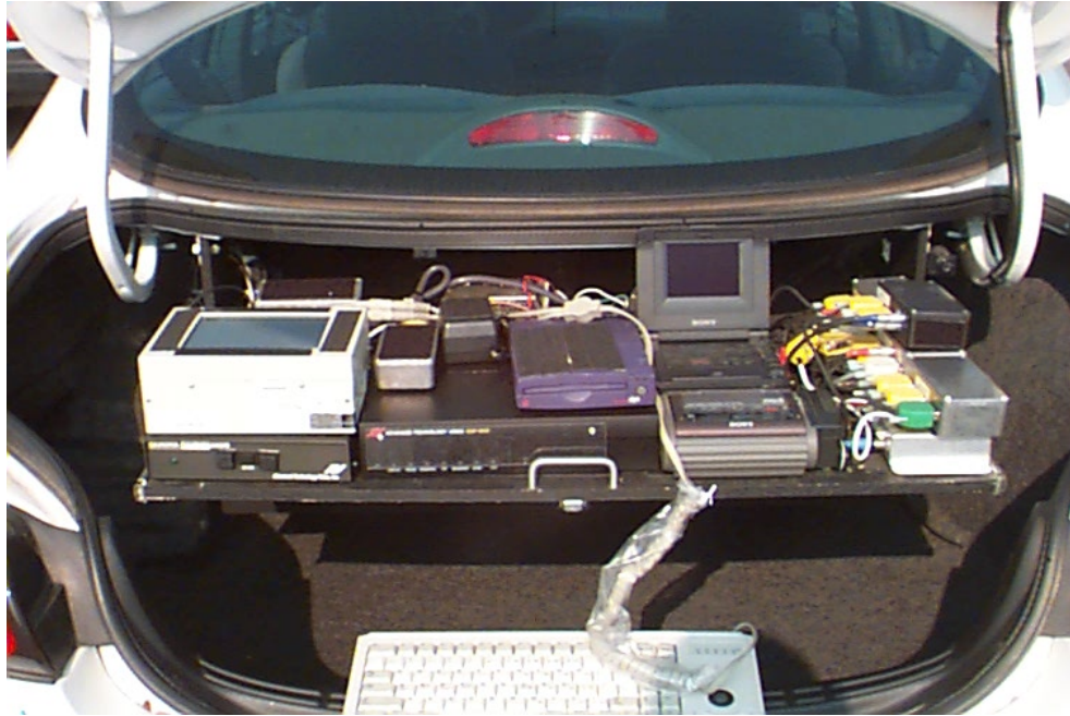
Figure 3.13. Data Collection Systems Storage Unit.
