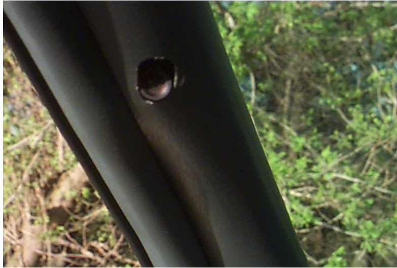
Figure 3.6. Driver's Face Camera Mounted within the A-Pillar.
