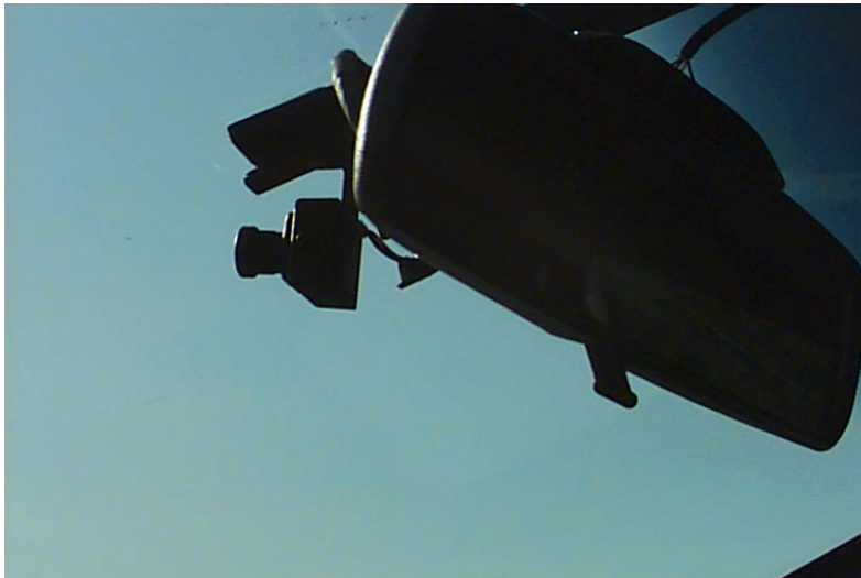
Figure 3.4. Forward View Video Camera Behind the Rear View Mirror.
