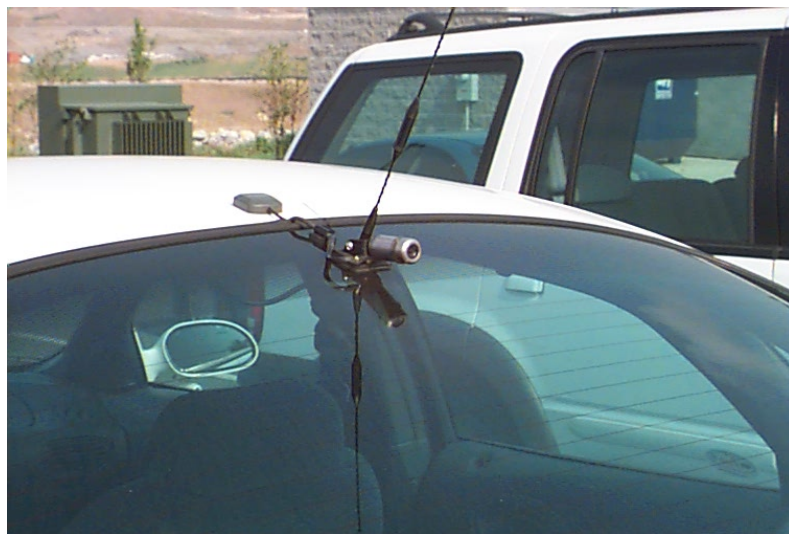
Figure 3.5. Rear View Video Camera Above the Rear Window.
