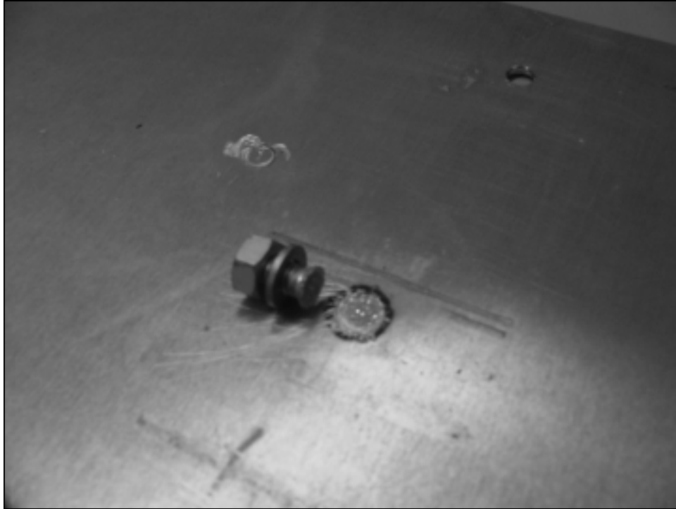
Figure 12. Failed Stud Due to Fatigue.
