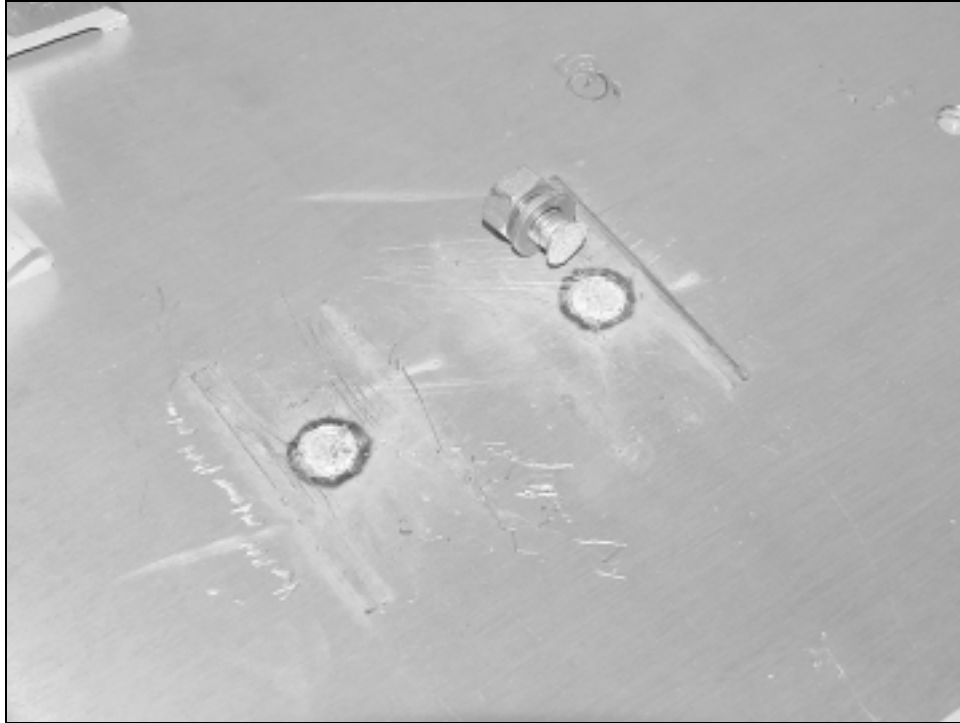
Figure 23. Failure of Weld.
