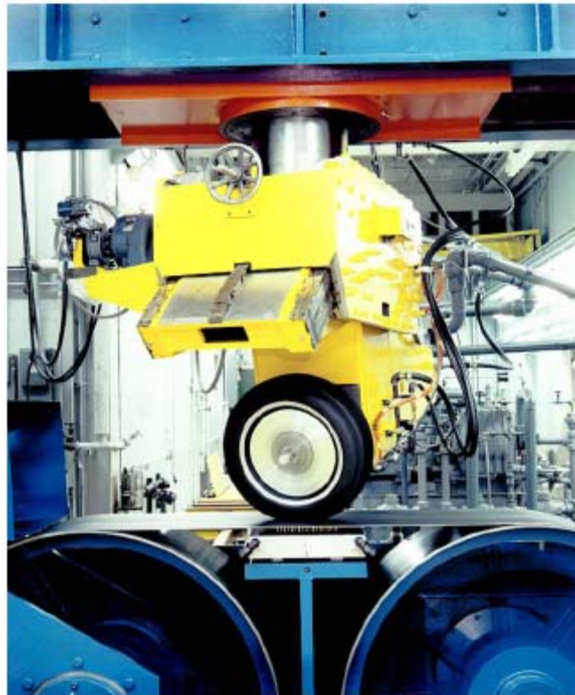
Figure 2.3. Calspan TIRF tire measurement machine [9]. Reprinted with permission from Calspan Corporation.
