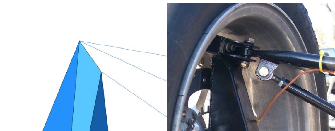
Figure 4.4. View comparing the pull rod mount in the Truss Model to a photograph of the same area from the completed 2009 VT-FSAE car.
