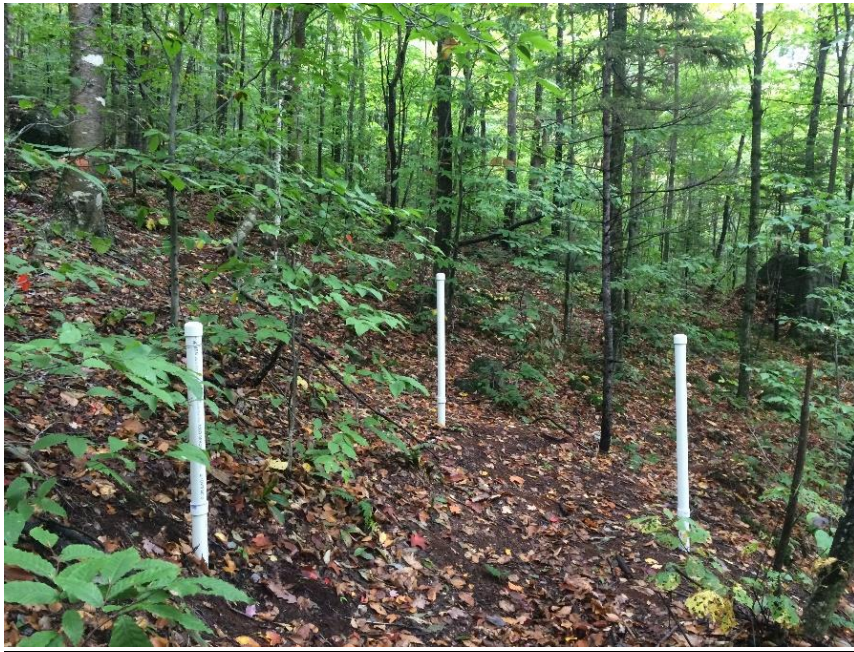
Figure 3: A cluster of shallow groundwater wells, (86)-4-c1, installed within the solum used for flow direction and hydraulic gradient calculations.
