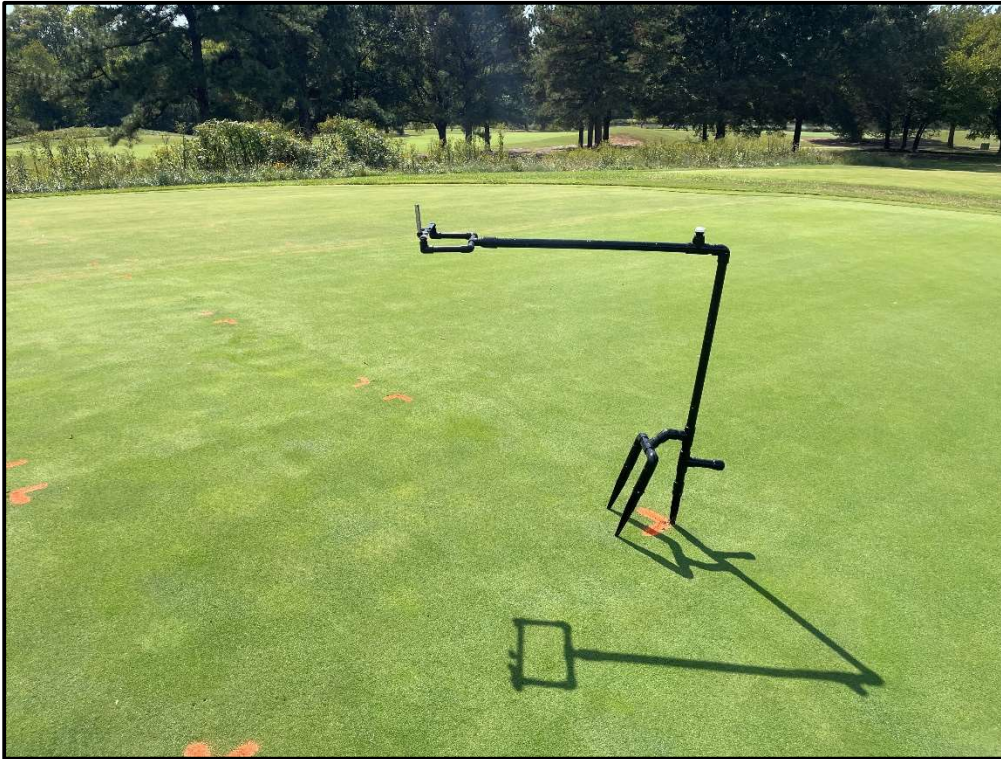
Figure 3. Representation of the custom-made PVC stand with a retrofitted arm that extends out 91.44 cm in length and holds the radiometer 5° field of view lens in order at a height of 127 cm to standardize the ground spectral data collection process at a spot sampling size of 10 cm 2 . This sampling standard was done for each location at the Pete Dye River Course in Radford, Virginia and The Country Club of Virginia in Richmond, Virginia.
