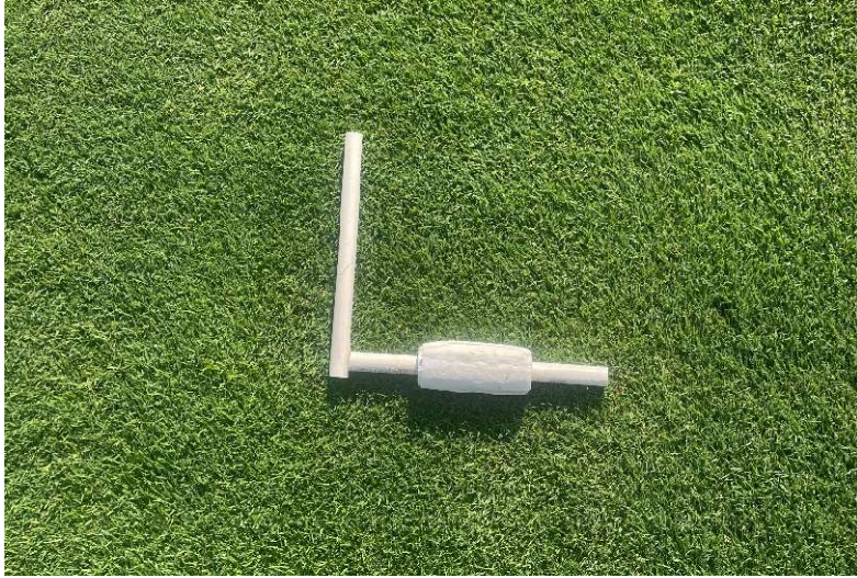
Figure 2. Visual example of the Custom PVC roller measuring 3.18 cm in diameter x 12.7 cm in length that has a smaller PVC handle inserted through the center and traversed across a length of 30.48 cm sampling a total area of 387.35 cm 2 on ‘Northbridge’ hybrid bermudagrass ( Cynodon dactylon x C. transvaalensis ) at the Country Club of Virginia in Richmond, Virginia.
