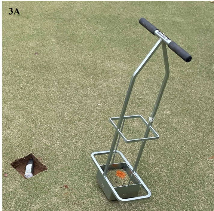
Figure 3. Illustrations showing the installation of the capacitive soil sensor using the Miltons square plugger on Green 9 in December 2022 at Independence Golf Club in Richmond, Virginia for (Figure 3A), a close-up of the capacitive soil sensor positioned horizontally before replacing the plug (Figure 3B), and the sensor in the hole rotated to ensure the moisture plate was perpendicular to the soil walls (Figure 3C).
