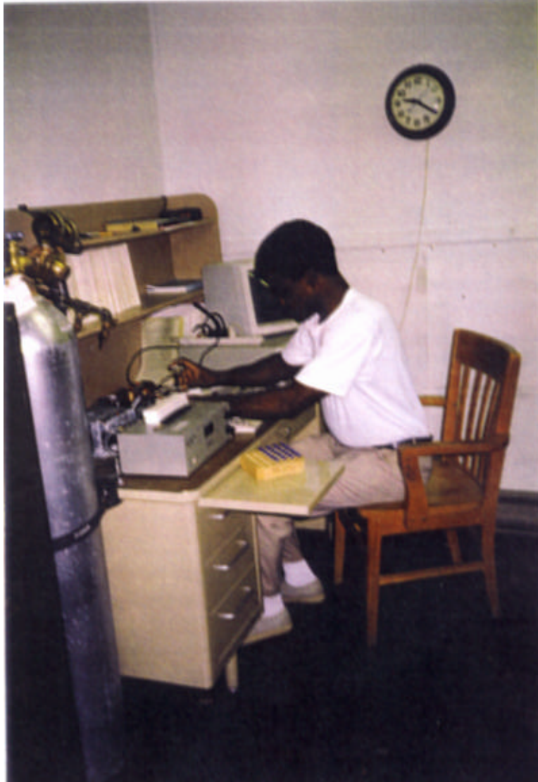
Figure C. Analyzing the samples of gas taken from the vials after temperature treatment for a pre-determined duration.
