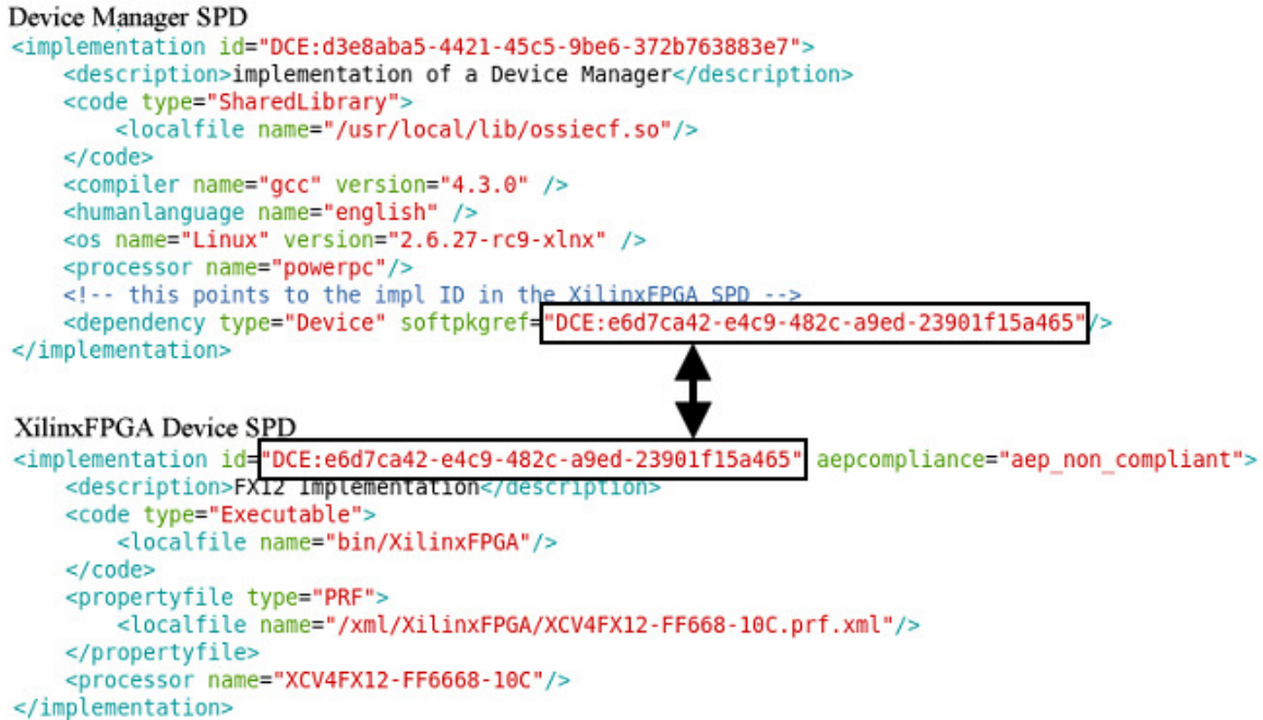
Figure 4: The SPD for the Device Manager must match the dependency UUID with the implementation id in the device SPD.
