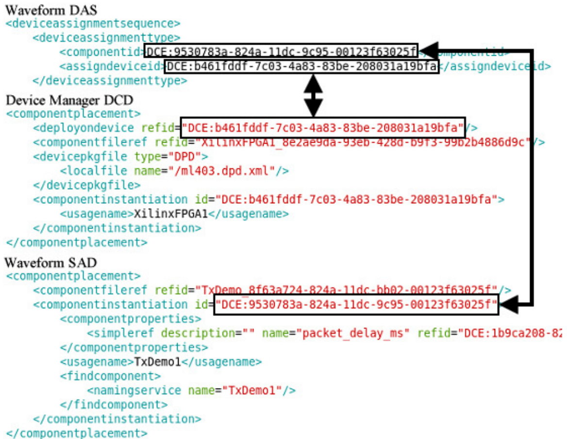
Figure 9: The DAS file uniquely links a component UUID to a node UUID. This example DAS file is from the ossie_demo waveform.
