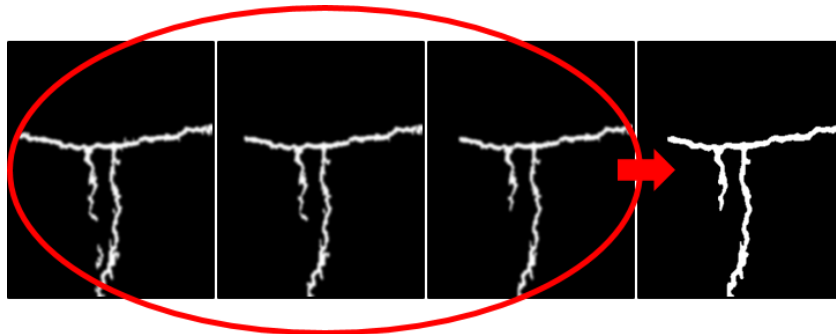
Figure 3.9: Correction in pre-processing: three crack PDFs corresponding to three different summation limits followed by final corrected image.
