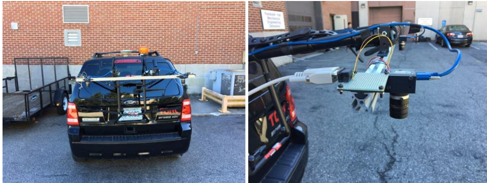
Figure 2.1: Car camera setup [51].
