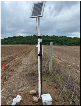
A do-it-yourself, low-cost, solar-powered spore trap sampler. Photo courtesy of Kamal Chhetri.
