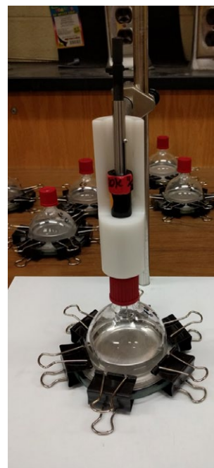
FIGURE 1 Reaction vessel used for aroma binding experiments
