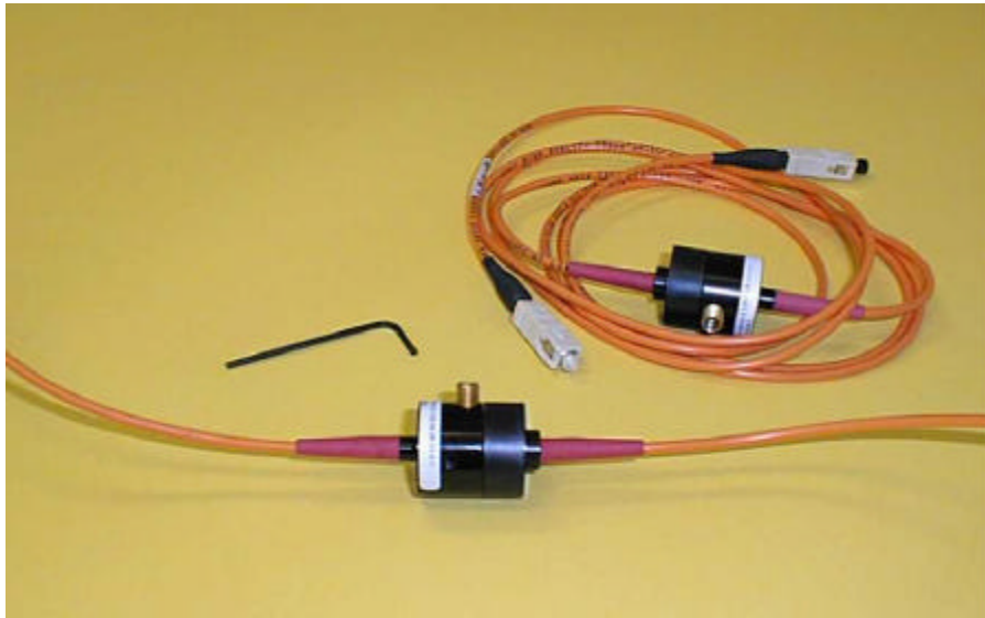
Figure 5.2 Variable Inline Attenuators Used between Ports on the ATM Switches
