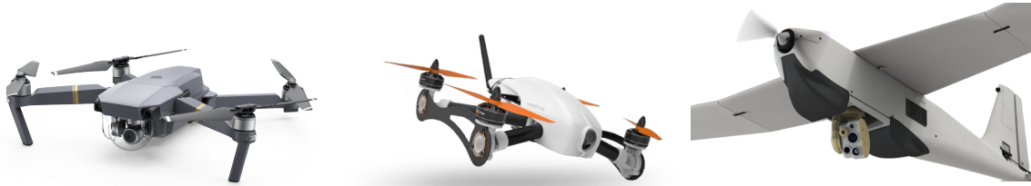
(a) A DJI Mavic Pro quadrotor UAV with great hovering endurance but lacks speed or efficiency compared to a multi-rotor UAV. (b) A Storm Racing Drone quadrotor UAV with great speed but lacks efficient hovering or endurance. (c) An AeroVironment Mantis fixed wing UAV with great speed and endurance but inefficient at station keeping compared to a multi-rotor UAV.
