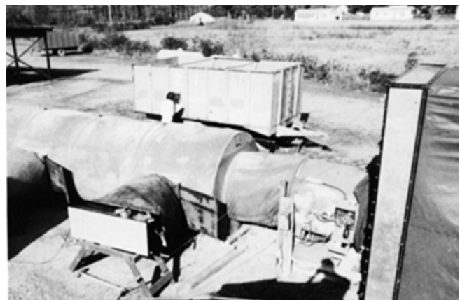
Figure 5. Use of calibrated resistance plates for on-farm testing of peanut dryer fans.
