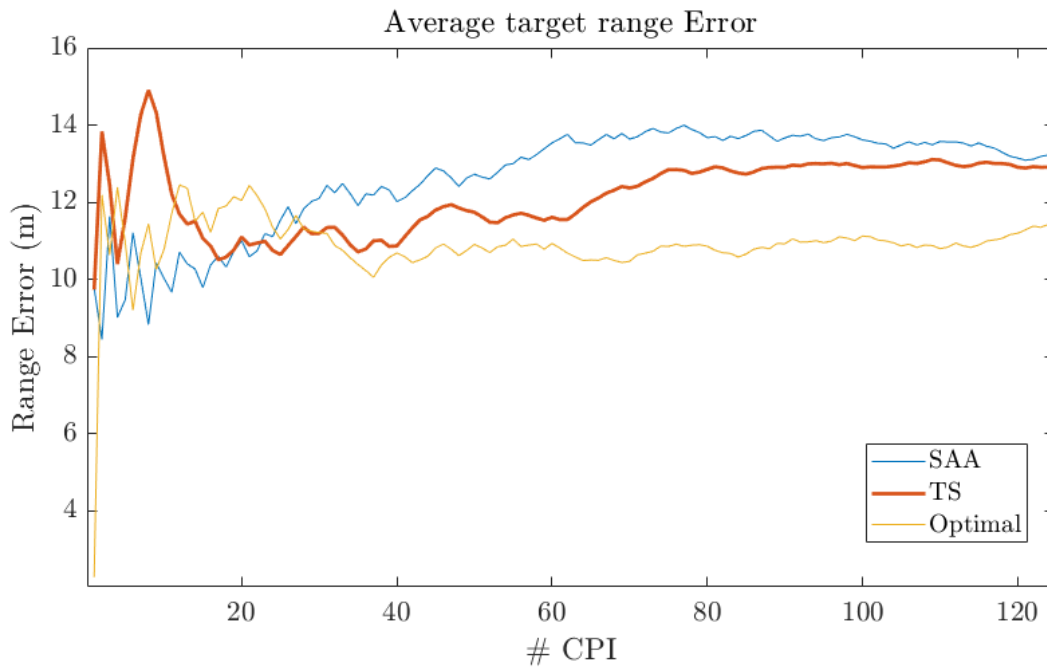
Figure 5.26: Average range error with a threshold set too high, incorrectly reporting subband 2.
