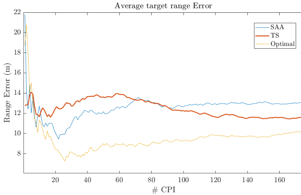
Figure 5.25: Average range error with a threshold set too low, incorrectly reporting subband 2.
