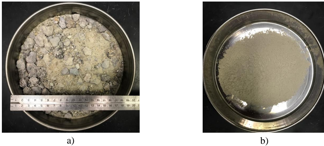
Figure 6- 2. SFS before (a) and after (b) processing by roller and ball milling.
