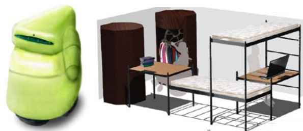
Figure 4. Concepts from the smart dorm course. Left: CARA, an assistive companion robot. Right: A modular furniture system that can be configured before the student arrives on campus via a survey system/virtual room builder application.
