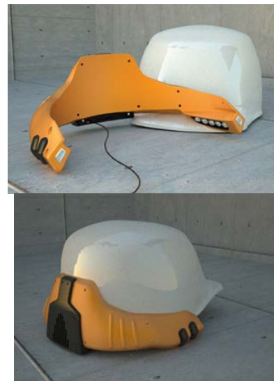
Figure 3. Digital rendering of hard-hat mounted active noise reduction concept.
