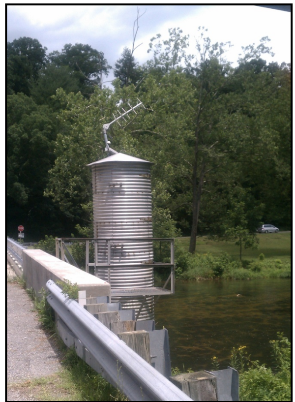
Stream-gaging station on Little River at Graysontown on the Montgomery Co./Pulaski Co. border, 7/15/12. Photo by Will Stacy.
